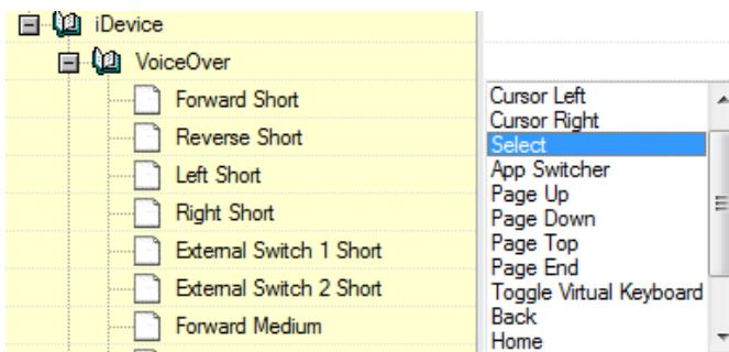
A total of twenty individual R-net commands can be used to control a connected iDevice. This is achieved using programmable Nudge Times which are applied to all four Input Device directions and switch functions. The Nudge Time parameters apply when using Switch Control or VoiceOver, giving a high degree of flexibility to cater for individual users' abilities. Additionally, the Speed Up and Speed Down buttons can be used as further control options.
